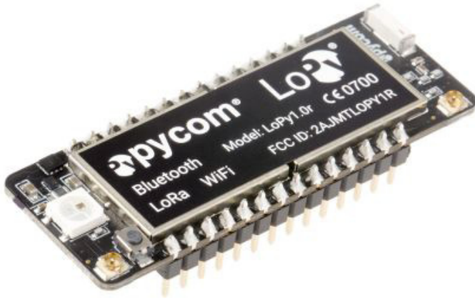
Figura 9. Tarjeta microcontrolador LoPy (Pycom, 2017)
